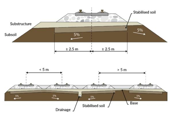
Figure 7.4 - Railway structure with stabilised layer
