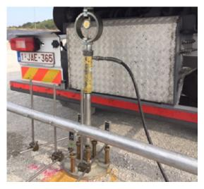
Figure 4.28 - Belgian plate test (© BRRC)
