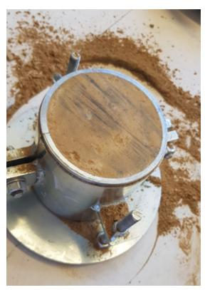
**Figure A1.11 –** Compaction mould (© Carmeuse)
