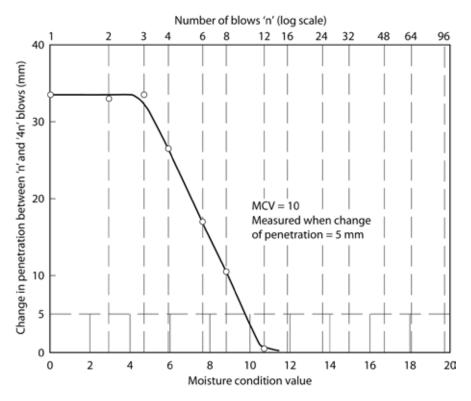
**Figure A1.15 –** MCV test (Parsons and Boden 1979)
