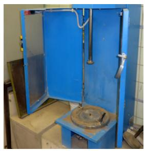
Figure A1.10 - Proctor equipment (© BRRC)
