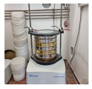
Figure A1.1 – Grading size equipment
