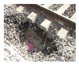
**Figure 7.3 –** Test pit showing contaminated ballast and a reinforced concrete slab at the bottom of the pit (Herle, 2005)
