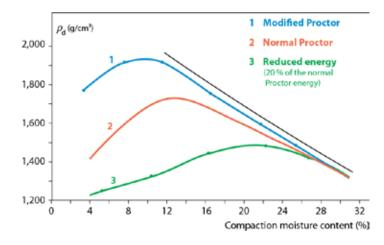
Figure 3.1a - Proctor curves (© BRRC)
