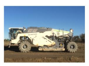
Binder spreader technology is also highly developed and can now very accurately spread the right amount of lime on the soil in accordance with the results of geotechnical studies performed by geo-laboratories. The long history of technology development, as well as the presence of major suppliers on all continents through their distribution networks, has inspired engineers, agencies and other stakeholders worldwide to design more and more projects that use soil treatment with lime for earthworks.
