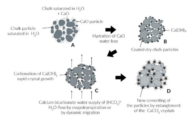
**Figure 7.24 –** Model of lime-treated chalk carbonation with the presence of bicarbonate ions in water (Paquet, 1993)
