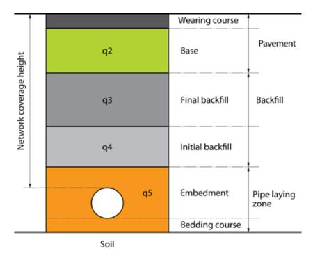
Figure 2.6 - Examples of compaction classes in France
