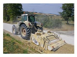
Figure 1.5 – Tractor-towed stabilisers for use in small-scale soil stabilisation projects (© Wirtgen)
