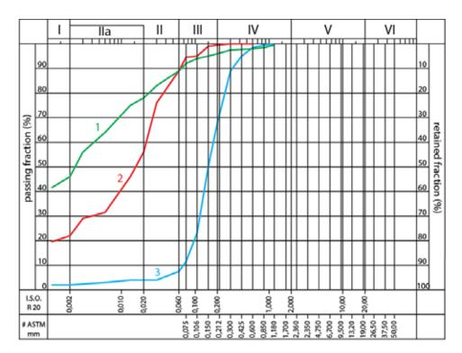
**Figure A1.3 –** Example of grading curves (© BRRC)
