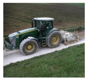
**Figure 4.17 –** *Tractor-towed stabiliser* (© Lhoist)
