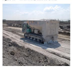
**Figure 4.11 –** Self-propelled spreading machine (© Lhoist)
