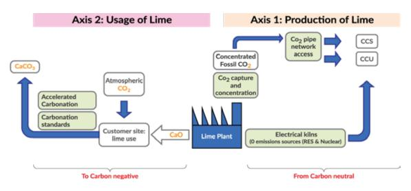
Figure 5.3 – Axes of work to reach net zero emissions by 2050 (© EuLA)
