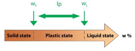
Figure 2.5 - Definition of plasticity index, liquid limit and plastic limit (© BRRC)
