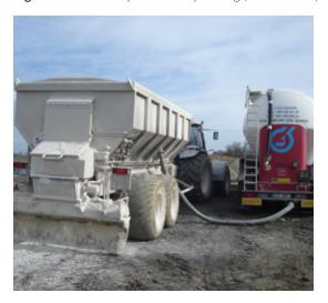
**Figure 4.10 –** Lime spreader with load transfer (© Lhoist)
