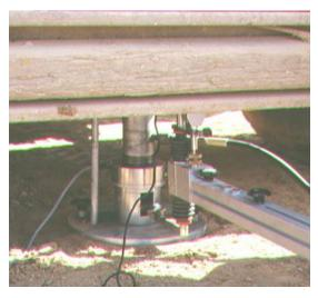
Figure 4.29 – German plate test (© Hessen Mobil)
