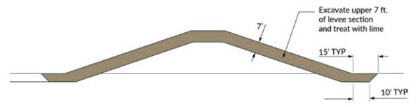
**Figure 7.13 –** Typical repair section of Mississippi levees (adapted from Forsythe, 1977)
