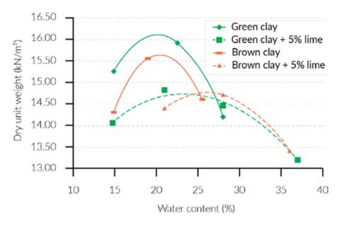
Figure 7.17 - Modified Proctor curves of untreated and treated clays
