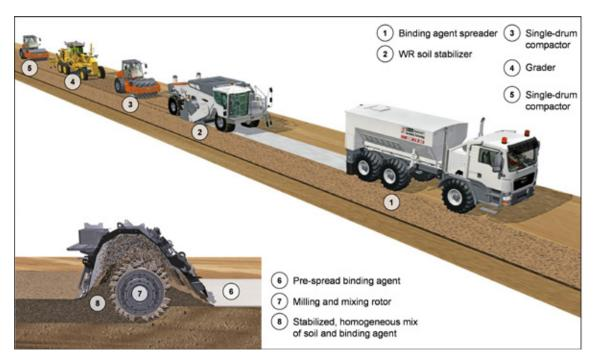
**Figure 4.1 –** Execution steps on the job site (© Wirtgen).
