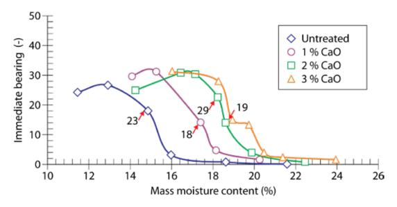
**Figure 2.10 –**  $I_{pp}$  curves of untreated and treated soil (Nguyen, 2015)
