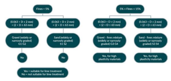
**Figure 2.1 –** Coarse and composite soils (D < 63 mm). This figure is based on EN 16907-2 (CEN, 2018b) 'Earthworks. Classification of materials.'
