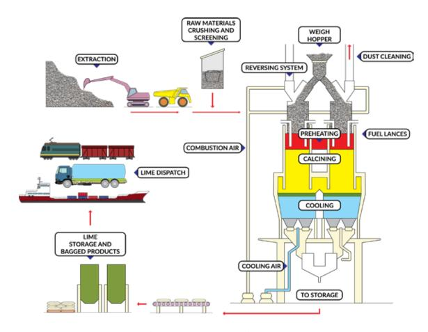
**Figure 5.1 –** Lime production process (British Lime Association, n.d.)
