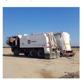
**Figure 4.4 –** Loading of large size spreader (© Carmeuse).
