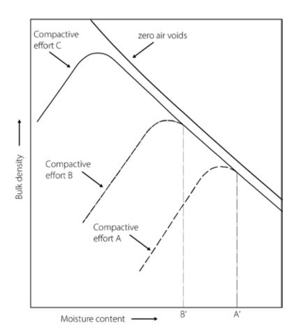
**Figure A1.13** - Relation between density and moisture content (Parsons & Boden, 1979)
