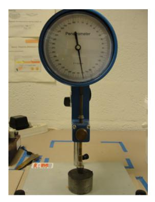
Figure A1.7 - Cone penetration test - liquid limit test (© Lhoist)
