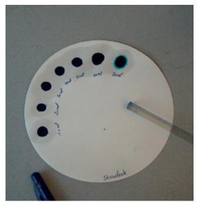
Figure A1.8 - Methylene blue test (© BRRC)
