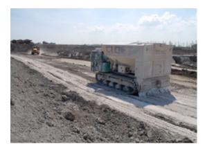
**Figure 1.4 –** Self-propelled spreading machine (© Lhoist)
