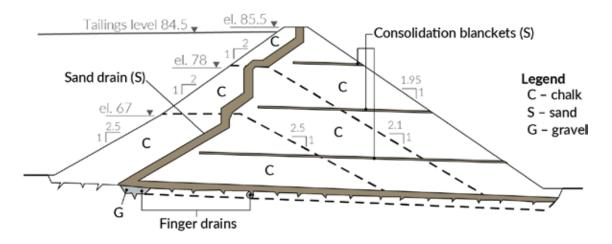
**Figure 7.27 –** Typical section of the chalk mud storage zone and dam
