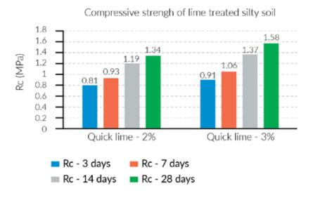
**Figure 7.22 –** Compressive strength measured at moisture content = 18% and 19%
