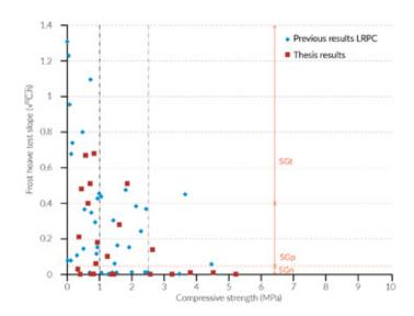
**Figure 7.10 –** Swelling slope versus compressive strengths
