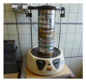
**Figure A1.2 –** *Grading size equipment (© BRRC)*
