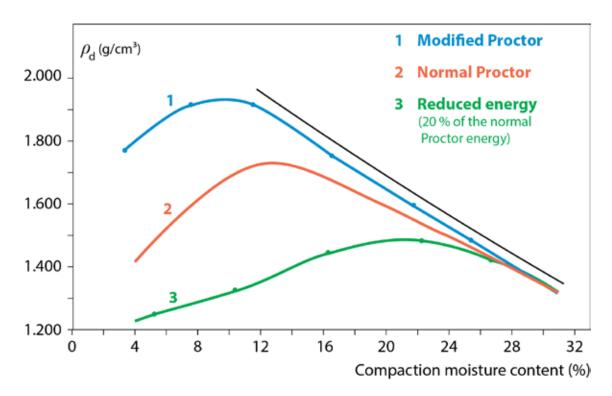
Figure A1.12 - Proctor curves (© BRRC)
