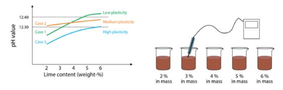
**Figure A1.19** – Practical example of lime fixation point determination
